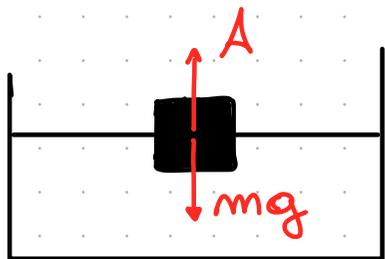
$$\Rightarrow T' = mg - A = mg - \rho_{H_2O} V_{imm} g$$
