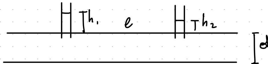
$$Q = v_m S = v_m \pi \frac{d^2}{4} \Rightarrow v_m = \frac{4Q}{\pi d^2} = 1,66 \text{ m/s}$$
