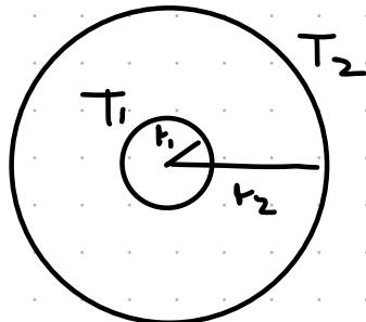
$$\text{MO} \quad dT = \frac{dQ}{dt} \frac{dx}{KA} = P \frac{dx}{KA}$$
