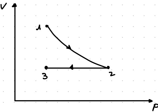
$$\text{d2: } W = m R T_1 \ln\left(\frac{V_2}{V_1}\right)$$
