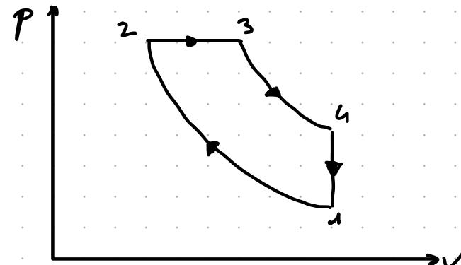
$$\text{H0} \quad Q_{23} = m c_p (T_3 - T_2) > 0 \Rightarrow Q_{23} = Q_{\text{ASS}}$$
