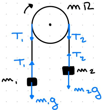
ORA TENGO CONTO CHE LA TENSIONE NON SARA' PROPAGATA LUNGO IL DISPOSITIVO, MA CI SARA' UNA TENSIONE TRA LA CARRUCOLA E CIASCUNA MASSA  $m_i$
