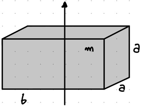
$$I = \int b^2 dm = \rho \int (\sqrt{x^2 + y^2})^2 dx dy dz = \rho \int_{-b/2}^{b/2} dx \int_{-a/2}^{a/2} dy \int_{-a/2}^{a/2} dz (x^2 + y^2)$$
